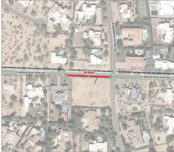
ID 663083 (Mountain View Rd. & Morning Glory Rd) 286 LF of 8" VCP
